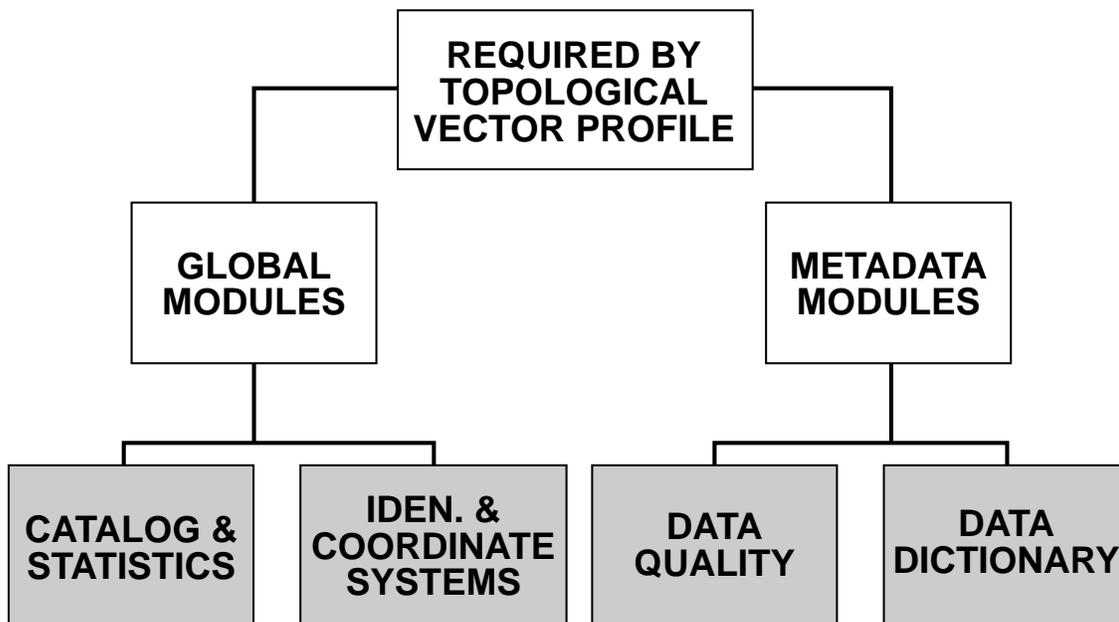
The modules that make up both global and metadata module categories must be present in all SDTS/TVP transfers.
